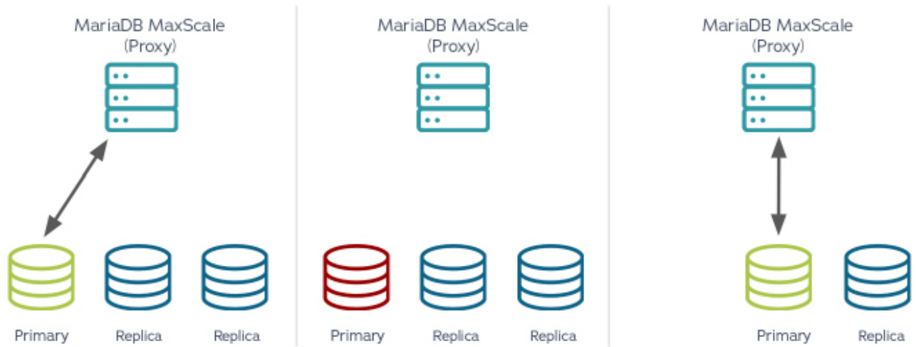
Diagram 3: Automatic failover with primary/replica replication
